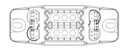
1 Begin with the Light Head and a Phillips Head Screw Driver. There are eight (8) Screws located on the front of the Protective Cover, and two (2) Screws on the top of the Light Head. Remove all ten (10) Screws from the Protective Cover.
