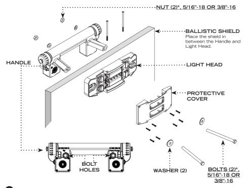
Begin by drilling two holes into the shield. To do this, locate the Bolt Hole(s) (2) located on the BACK SIDE of the Handle (shown above).
