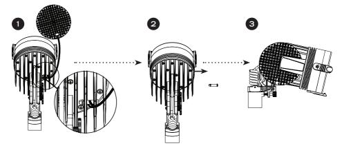
Press the retaining fastener through the heatsink fins, laterally. The spring end will compress allowing it to fit through the hole.
