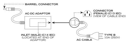
The plug of the AC Cable should be country specific. Example: IEC Types A-N. The Female Connector side of the AC Cable must be IEC Type C13 to mate with the Male Inlet of the AC-DC Adaptor.
