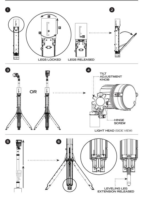
1 Set the Nomad<sup>®</sup> down vertically, on a flat surface, as shown. Open the Protective Light Cap and twist the Locking Sleeve to the right (A) and slide upwards (B). While still holding the Locking Sleeve up, twist it back to the left (C). The folding Tripo-Scope<sup>®</sup> Legs are now accessible to deploy (D).
