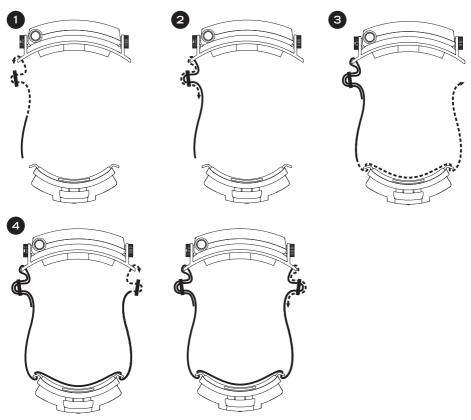
Place the headlamp on a flat surface. Position the Light Head so the Power/ Mode Switch is on the left and the LEDs face forward. NOTE: Make sure the FoxFury logo on the Battery Pack is correctly oriented before beginning.
