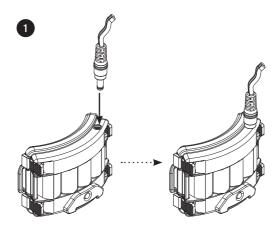
Begin by plugging the AC-DC Adaptor into an outlet. The Charge Indicator will then turn solid green.
